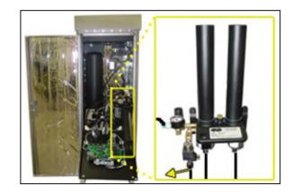
**9.7.4** Place your hand beneath the Unloader Valve fitting to feel for air flow.
