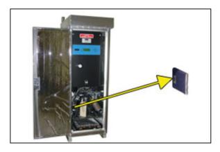
**6.6.5** Remove the shipping block from under the compressor plate.
