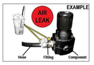
If any leaks are detected, take steps to seal them off (as necessary):
