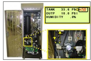
When the compressor runs for 3:00 minutes (unless adjusted to a different Set Point by the user), a Compressor Excessive Run Time (**LAST RUN**) alarm should appear on the System Screen.
