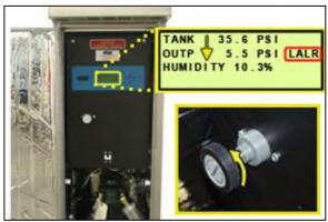
After one (1) minute, the Low Pressure Alarm should appear on the display.
