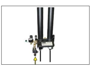
If air flows from this valve continuously the Unloader Valve is defective and should be replaced. See sections 11.3 for part detail and 11.7 for ordering information.
