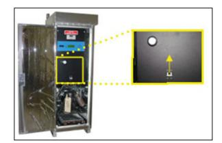
**IMPORTANT:** Press **RESET** if the dryer goes into **SHUTDOWN** due to Humidity.
