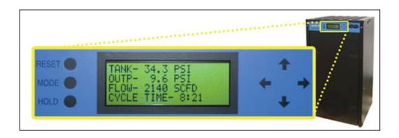
**8.4.1 RESET Button** – Clears an alarm and allows the system to continue operating.
