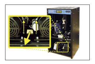
**6.5.6** Remove the ship-loose contents package.
