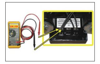
The voltage should measure 106 Volts DC.
