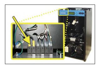
9.4.3 Place Voltmeter probes between the Circuit Breaker and terminal insulation so that they touch the metal contacts.
