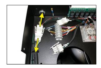
**6.5.13.4** Plug both of the Boost Transformer Lead connectors into the Main Power Lead connectors.
