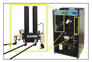
**9.7.3** Place your hand beneath the Unloader Valve fitting to feel for air flow.
