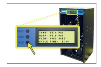
**9.15.3** Make a note of the current Outlet Pressure (**OUTP**) reading.
