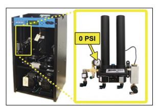
**9.13.5** Unscrew and remove the Humitter from the Humidity Block.
