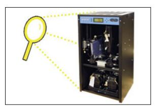
**6.5.5** Remove the shipping block from under the compressor plates.
