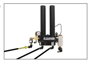
If air flows from this valve continuously the Unloader Valve is defective and should be replaced. See sections 11.3 for part detail and 11.7 for ordering information.
