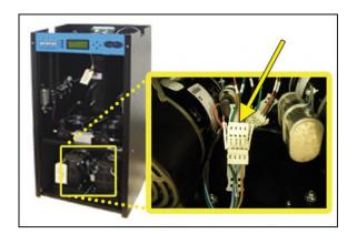
9.3.3 Use a Voltmeter to measure the voltage between the Hot and Neutral wires by placing the probes in the openings in the power connector:
