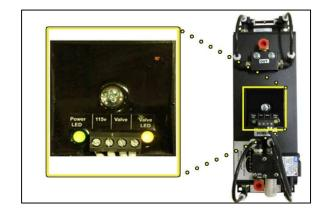
If either light is off see sections 8.3 and 8.4 to verify the cycle timer has correct voltages.
