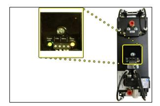
The second set is the 4 Way Valve and is labeled "Valve".
