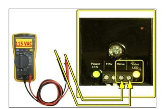
Continue to measure for up to 90 seconds if no voltage is initially measured.
