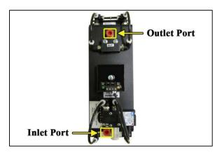
**6.5.5** Install inlet and outlet fittings, filters, and/or assemblies to air dryer.
