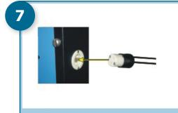
• Insert the Power Fail Alarm Plug into the Power Fail Alarm Socket.
