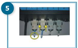
Attach and secure the DB9 cables routed from the dryers, starting with #1 on the left.
