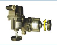
• Turn the Bypass Valve (in back) clockwise until it is completely closed.
