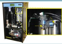
• Unlock the Bypass and Back Pressure Valve knobs by loosening the retaining nuts.
