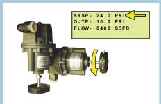
Adjust the Bypass Valve (in back) until the **SYSP** reading on the Front Panel Display equals the Bypass Pressure value determined earlier in this Step.
