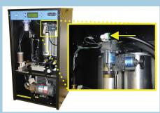
• Re-connect the Back Pressure Tube by pressing it firmly into the green ferrule.
