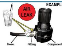
If air bubbles appear, this is an indication that air is leaking.
