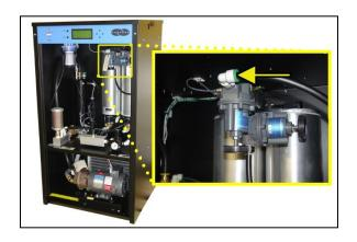
**8.11.1.9** Open the Bypass Valve until the **SYSP** reading on the front panel display is correct according to your elevation. (see chart 8.11.1)
