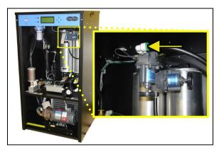
**8.11.1.9** Open the Bypass Valve until the **SYSP** reading on the front panel display is correct according to your elevation. (see chart 8.11.1)
