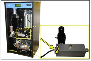
9.15.10 Press the RESETButton to clear the Humidity alarm.
