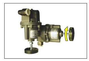
**6.5.23.5** Push the Back Pressure Tube in and hold the green ferrule. While holding the ferrule pull the tube out.
