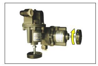
8.11.1.6 Push the BackPressure Tube in and hold the green ferrule.While holding the ferrule pull the tube out.
