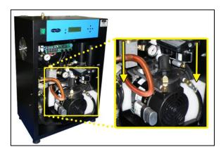
**6.5.6** Remove the Plug from the Outlet Port by pressing the ferrule down then pulling the plug upward.
