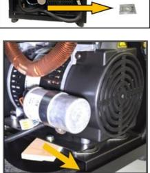
**6.5.6** Remove the Plug from the Outlet Port by pressing the ferrule down then
