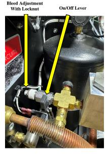
enables (inline position) or disables (perpendicular position) its operation and the bleed adjustment with locknut which allows you to precisely adjust the amount of air being bled out of the tank.
