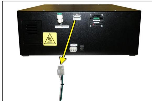
**9.2.2.2** Place Voltmeter probes inside the DC Power Harness connector socket:
