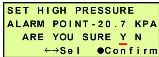
**8.8.2.6** Press the Function (●) Button to Confirm. This will lock in the new setting value.
