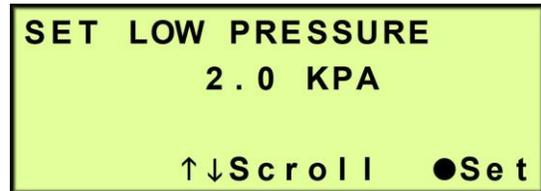
**8.7.5.2** Press the Right (→) & Left (←) Arrow Buttons to move the underscore beneath the digit to change.
