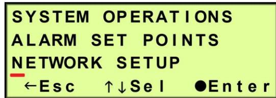
**6.5.17.2** Press the Function (●) Button to Enter Network Setup.
