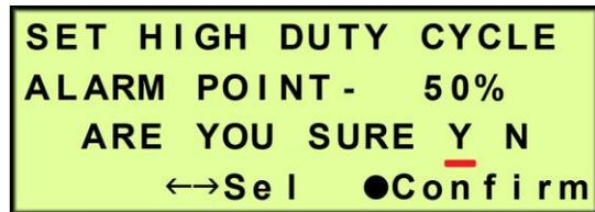
**8.8.12.6** Press the Function (●) Button to confirm. This will lock in the new setting value.
