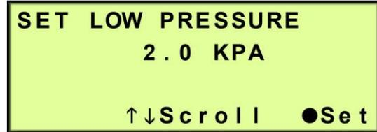
**6.5.15.2** Press the Left (←) & Right (→) Arrow Buttons to move the underscore beneath the digit to change.
