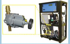
• Unlock the knob on the System Pressure Regulator by loosening the retaining nut with a 1/2" wrench.
