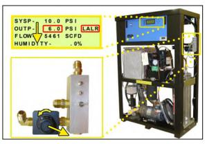
After one (1) minute, the High Pressure Alarm should appear on the display.
