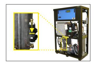
**9.13.9** Reinstall Inlet Air Filter Assembly.
