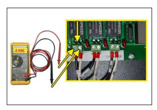
9.10.7 Use a Voltmeter to measure the AC voltage across the terminals "Heater2" wire #30 BLK & #16 WHT.
