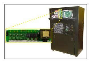
9.10.6 Use a Voltmeter to measure the AC voltage across the terminals "Heater 1" wire #29 BLK & #15WHT.
