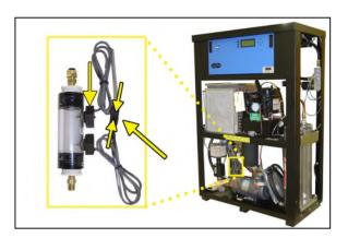
**9.14.4** Remove the Inlet Air filter.
