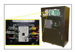
9.16.3 Use a Voltmeter to measure voltage to "L" Side of the Power Contactor.
