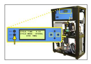
**8.4.6.3** Press the Left (←) Arrow Button to increase the hour value of the cycle time.
