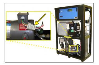
**9.2.3** Use an Amp Meter to measure the running amps for the compressor.
