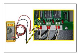
9.9.12 Use a Voltmeter to measure the DC voltage across the terminals "Tower2" wire #28 BLK & #19WHT.
