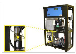
9.13.4 Keep adding water until the water level is above the Dump Water Sensor and the Dump LED is lit.
