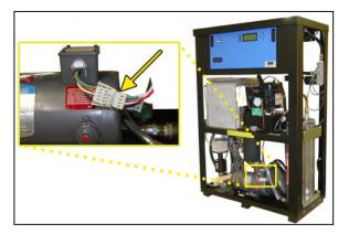
**9.3.3** Use a Voltmeter to measure the voltage.
