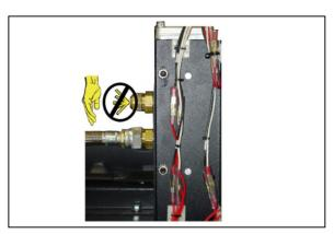
9.8.9 Using a 1-1/4" wrench completely disconnect the Bottom Braided Hose from the 4-Way Valve Assembly.
