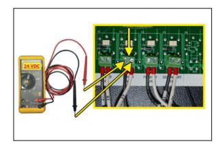
The voltage should measure **24 Volts DC**
