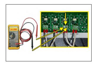
The voltage should measure 24 Volts DC.
