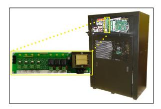
**9.9.6** Use a Voltmeter to measure the DC voltage across the terminals "**Tower 1**" wire #27 **BLK** & #18 **WHT**.
