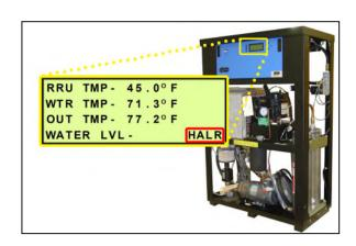
9.14.11 The dryer will dump the water until it stabilizes just below the High Water Sensor, and the High Sensor LED will turn off.
