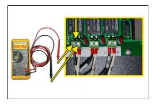
9.10.12 Use a Voltmeter to measure the AC voltage across the terminals "Heater2" wire #30 BLK & #16WHT.
