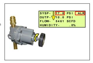
After one (1) minute, the Low System Pressure Alarm should appear on the display.
