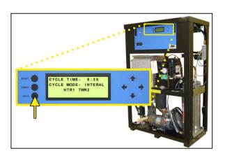
**9.9.2** Make a note of the current **CYCLE TIME** reading.
