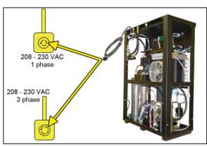
**NOTE:** ALTEC AIR recommends using a 20 amp 250 VAC plug. (not provided)
