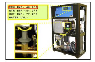
**8.15.5** Allow the unit to run for at least 45 minutes to reach equilibrium. **NOTE:** If after 45 minutes the **RRU TMP** on the display does not stabilize between 35° - 45°F, repeat steps 8.15.4
