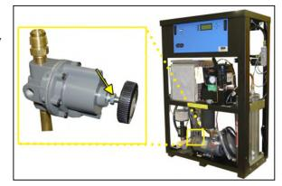
9.7.5 Turn the System Pressure Regulator counter-clockwise until the SYSP reading on the Front Panel Display is below 18.0 PSI.
