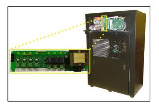
9.13.7 Use a Voltmeter to measure voltage to PrimaryDump Solenoid while dryer is dumping water.
