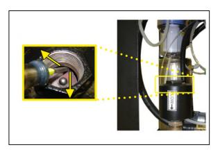
**6.5.20** Reinstall Inlet Air Filter assembly.
