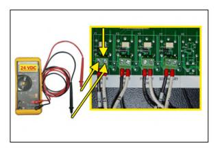
9.9.7 Use a Voltmeter to measure the DC voltage across the terminals "Tower 2" wire #28 BLK & #19 WHT.
