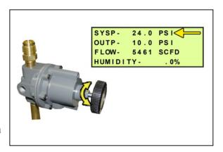
**6.5.25.4** Lock retaining nut on the System Pressure Regulator.
