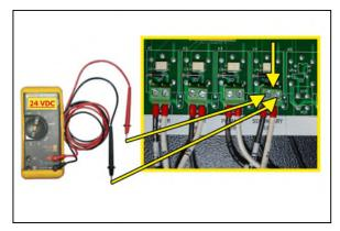
The voltage should measure 24 Volts DC.
