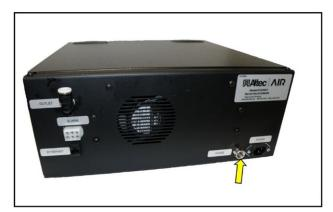
• Place your hand behind the purge port to feel for purging air. Air should be steadily purging from the port, and a burst of air should be felt every 60 seconds as the dryer cycles between towers.
