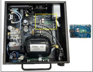
**9.4.3** Use a Voltmeter to measure across the board terminals where wires #4 and #5 are connected.
