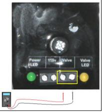
If the voltage does not measure approximately the same as the incoming system voltage the Cycle Timer could be defective. See sections 11.2 for troubleshooting information.
