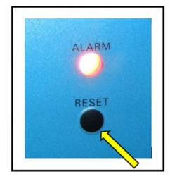
**9.11.6** Press the **RESET Button** to clear the alarm.
