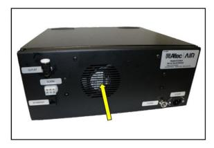
**NOTE:** Fan will turn OFF when the cabinet temperature is below 80° F (27° C).
