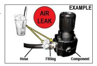
If any leaks are detected, take steps to seal them off (as necessary):
