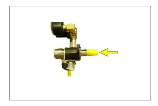
If air flows from this valve continuously the Unloader Valve is defective and should be replaced. See sections 11.3 for part detail and 11.8 for ordering information.
