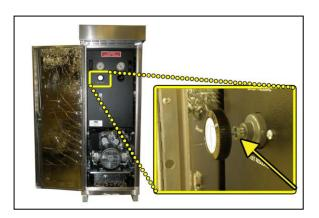
9.15.4 Turn knob until OutletPressure reading is below 6.5PSI (unless adjusted to a different Set Point by the user).
