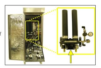
**9.8.4** Use a Voltmeter to measure the DC voltage across each set of "53VDC" terminals.
