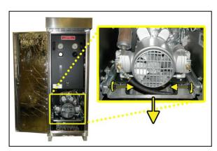
**6.5.7** With a 7/16" wrench remove the shipping blocks from under the compressor plate.
