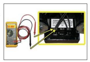
The voltage should measure 53 Volts DC.
