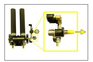
**9.7.4** Place your hand behind the Unloader Valve fitting to feel for air flow.
