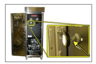
**8.10.3** Turn knob until Outlet Pressure reading is at the desired alarm setting.
