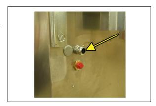
**6.5.14** With a 5/16" nut driver, remove the cover from the terminal block.
