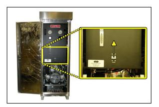
IMPORTANT: Press RESET if the dryer goes into SHUTDOWN due to Humidity.
