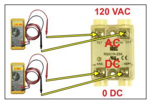
If any of the voltage measurements are different than indicated above, the Solid State Relay is defective and should be replaced. See sections 11.2 for part detail and 11.8 for ordering information.
