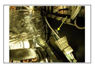
9.2.4 Use an Amp Meter to measure the running amps.With the compressor running, the running amps should measure
