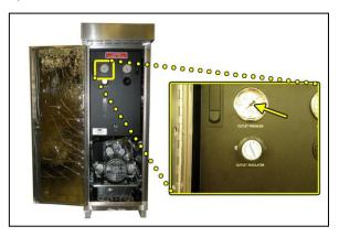
**9.15.3** Loosen the Outlet Pressure Regulator Locknut.
