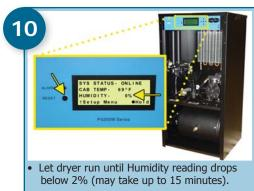
**NOTE:** Press **RESET** if the dryer goes into SHUTDOWN.
