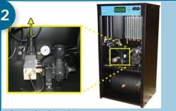
Power the dryer **ON**. Set the Static Pressure: • Pull Static Pressure Regulator knob out.
