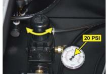
Adjust knob until reading on Pressure Gauge is 20 PSI.
