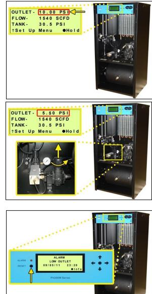
9.15.7 Turn Outlet Pressure Regulator knob clockwise until Outlet Pressure (OUTLET) reading raises to the reading recorded in step 9.15.1
