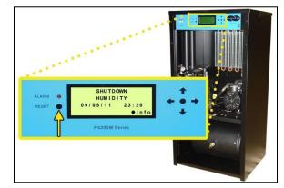
**NOTE:** If the Humitter is disconnected from the Control Board, **\*\*%** will appear on the Humidity reading and after 5 minutes the unit will Shutdown. This is to allow for troubleshooting.
