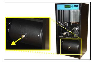
**9.13.4** Unscrew and remove the Humitter from the Combo Block.
