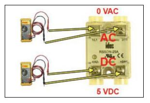
**9.5.5** Use a Voltmeter to measure across the AC terminals.
