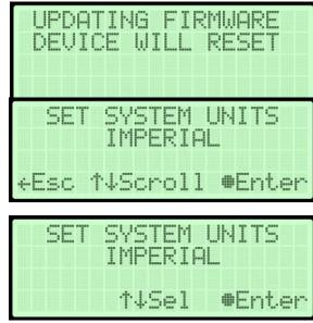
8.5.2.5 Press the Enter (●)Button to confirm the selected choice. This will lock in the new setting.
