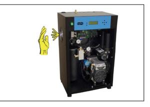
**NOTE:** The fan will turn OFF when the cabinet temperature is below 80°F (27°C).
