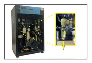
**9.11.3** Unscrew and remove the Humidity Sensor from the Humidity Block.
