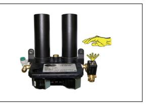
If air flows from this valve continuously the Unloader Valve is defective and should be repaired or replaced. See sections 11.3 for part detail and 11.6 for ordering information.
