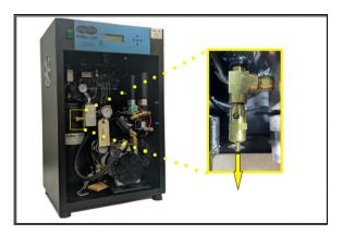
9.9.4 Verify the compressor turns on when the tank pressure (TANK) falls to 20.0 PSI (137.9 KPa).
