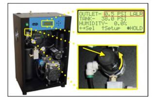
9.13.3 Turn Outlet Pressure Regulator knob clockwise until Outlet Pressure (OUTLET) reading rises to the reading recorded in step 9.13.1
