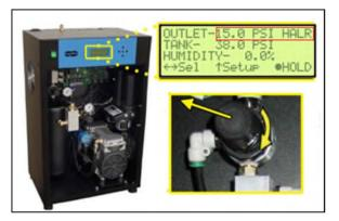
After one (1) minute, the High-Pressure Alarm should appear on the display.
