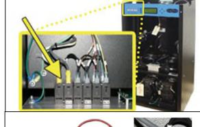
6.5.12.2 Use a Voltmeter to measure the voltage by placing the probes between the Circuit Breaker and terminal insulation so that they touch the metal contacts.
