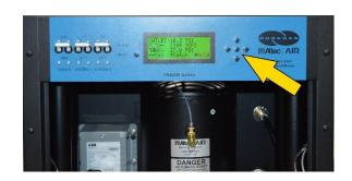
**9.15.3** Make a note of the current Outlet Pressure (**OUTP**) reading.
