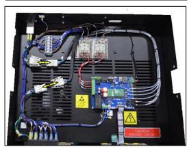
**6.5.13.4** Plug both Boost Transformer Lead connectors into the Main Power Lead connectors.
