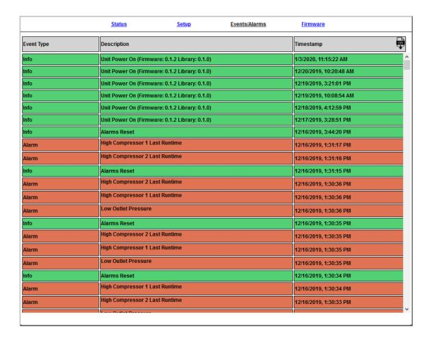
Displays all events such as alarms, changes made, and alarm resets registered by the P8400W Series Air-dryer. This screen is informational only. You may download a .csv file with all event/alarm information by clicking on the "Download CSV" button at the top right hand corner of the table.
