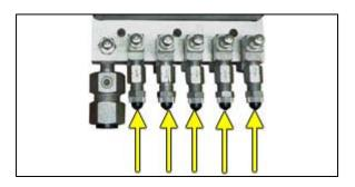
**6.5.5** Use a flathead screwdriver to Open / Close the Outlet Ports as required:
