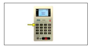
**6.4.5** Power OFF the PVD860D and remove test pair.
