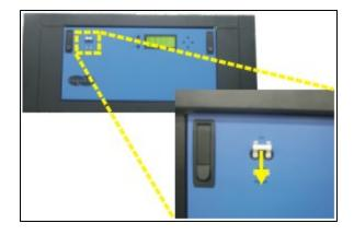
2. Install PVDW31 interface module onto the back of the front panel as shown.
