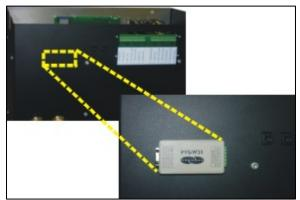
4. Install and route the interface cable as shown.
