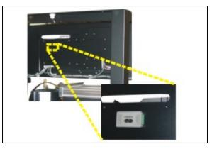
3. Attach the end of the interface cable to the PVDW31 Ty-rap as needed. Route as shown.
