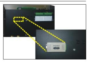
4. Install strain relief around interface cable and route cable into the unit. Install strain relief into hole. Attach the other end of the interface cable to the PVDW31 Ty-rap as needed.
