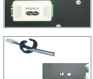
Locate the 25' DB9 cable and the cable markers. Label both sides of the cable with the desired marker number. Connect the cable to the DB1 of the PVDW31 module. Route the other end to the P08033W Cycle Module, but do not connect to the cycle module. (See cycle kit installation guide).
