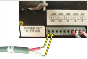
13. Route cable **C** through the air dryer and install into the reset switch.
