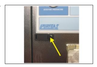
3. Locate the two black latches holding the acrylic cover on. Unlatch and bring down the acrylic cover.
