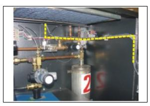
15. Remove the two wires from the reset switch on the air dryer.
