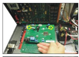
11. Remove the two wires from the reset switch on the air dryer.
