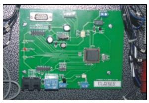
8. Reinstall wires A and B into P1 of the PVDW33 board.
