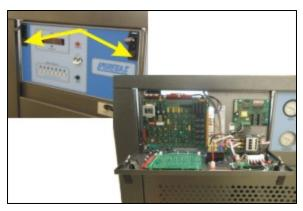
3. Remove the two screws holding the plastic clamps on the display board.
