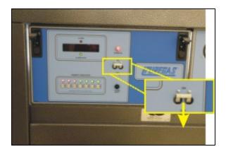
2. Release the latches and lower the front panel.
