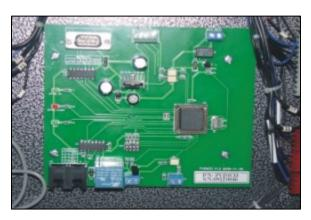
6. Connect the 4-pin cable(supplied) from P5 of the PVDW33 board to the W9 connector of the alarm board of the dryer.
