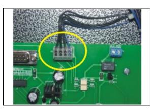
11. Locate the 25' DB9 cable and the cable markers. Label both sides of the cable with the desired marker number. Connect the cable to the DB1 of the PVDW33 module).
