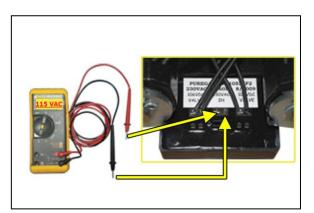
If the incoming voltage measures less than indicated above, it is recommended that steps be taken at your facility to increase the incoming power to the recommended levels. **8.3.4** Reinstall the Manifold Cover.
