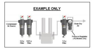
**CAUTION**: When installing a typical Complete Air Dryer, or Point-of-Use System, Altec AIR recommends assembling ALL components before mounting the VSA Series Air Dryer.
