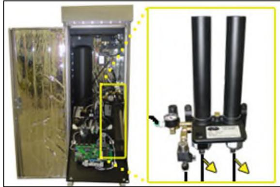
**9.6.4** Place your hand beneath the purge fittings to feel for purging air. Air should:
