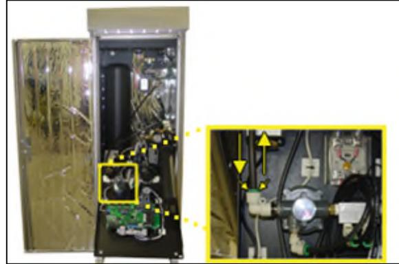
**8.9.4** To prevent pressure from building back up, power the dryer **OFF** (*See 8.3 section for detail*).
