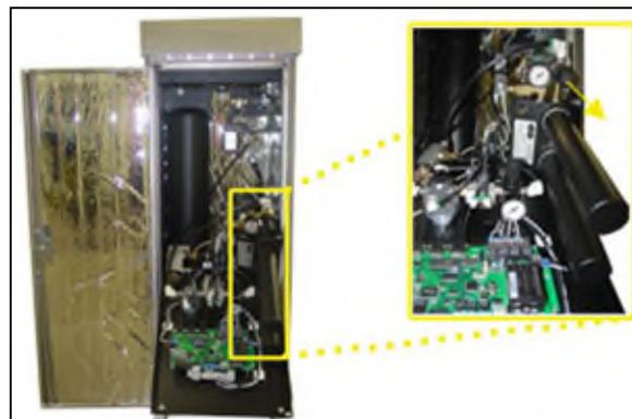
**8.10.4** Turn the knob until the reading on the Pressure Gauge is **50 PSI**.
