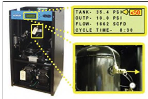
When the compressor(s) runs for 3:00 minutes (unless adjusted to a different Set Point by the user), a Compressor Excessive Run Time (**LAST RUN**) alarm should appear on one or both of the System screens.
