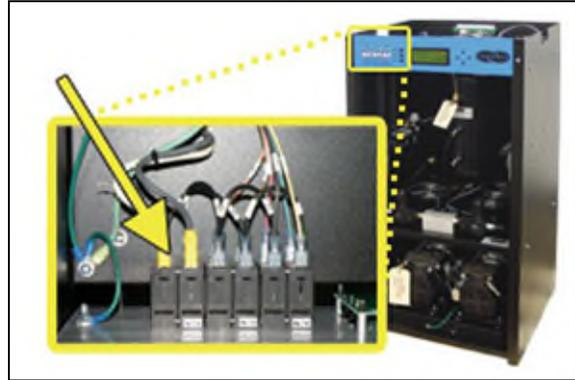
**6.5.12.2** Use a Voltmeter to measure the voltage by placing the probes between the Circuit Breaker and terminal insulation so that they touch the metal contacts.
