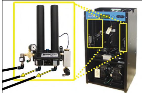
**9.6.3** Place your hand beneath the purge fittings to feel for purging air. Air should:
