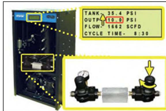
**9.15.8** Press the **RESET Button** to clear the alarm.
