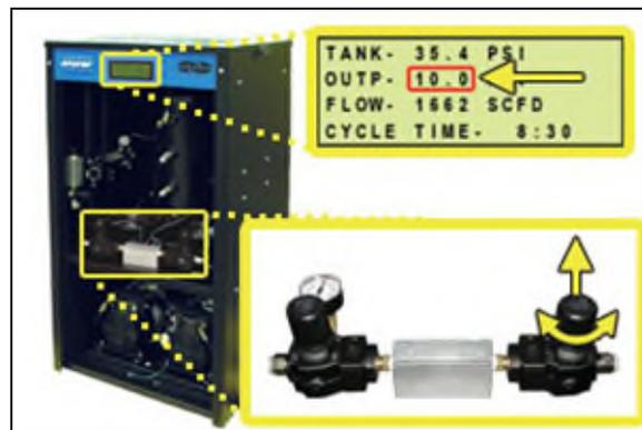
**6.5.22.3** Turn knob until Outlet Pressure (**OUTP**) reading is at the desired setting.
