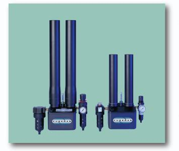
Compact, regenerative CO extractors capable of delivering up to 5.4 SCFM at 100 PSIG of dry, CO-free air, with a dewpoint of -40°F (-40°C) and a CO content of less than 2 ppm. Ideal for emissions monitoring applications. Units come standard with a moisture indicator. Accessories include an inlet particulate filter, inlet coalescing filter, outlet filter-regulator assembly, flow meter, surge tank, wall-mount bracket and sound suppression kit.
