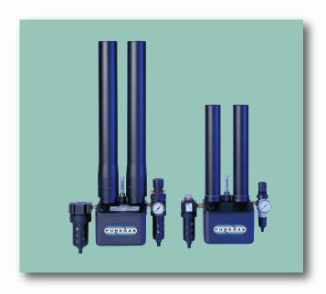
Compact, regenerative hydrocarbon adsorbers capable of delivering up to 7.5 lpm of air with a hydrocarbon content of less than 1 ppm. Designed for GC-FID and emissions monitoring applications. Accessories include an inlet particulate filter, inlet coalescing filter, outlet filter-regulator assembly, moisture indicator, flow meter, surge tank and sound suppression kit.
